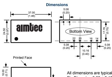
4.10 (0.16) All dimensions are typical: millimeters (inches) Pin Diameter:  $0.60 \pm 0.10 (0.02 \pm 0.004)$ Case Tolerance:  $\pm 0.5 (\pm 0.02)$
